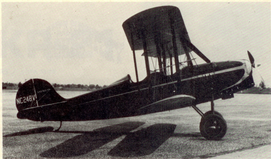
Fitted with the 135-hp Ranger, the two KR-135s reverted to the wing and landing gear configuration of the KR-21A. Lettering on the fin indicates that this example is being demonstrated as the Pilgrim 135 of The American Airplane and Engine Corp., not as a Fairchild.
